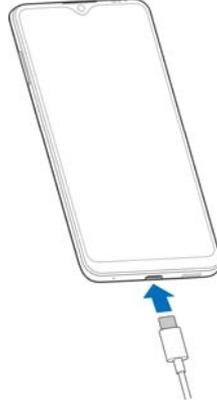
2. Connect the charger to a standard AC power outlet.
